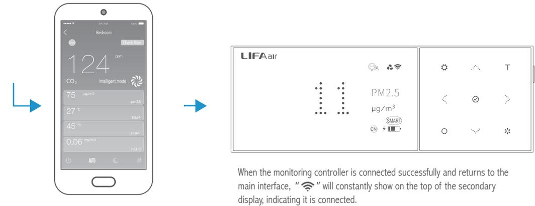
Note: To control main unit via phone and to read data such as temperature, humidity, filter life-span etc. the monitoring controller must be connected to the main unit.
