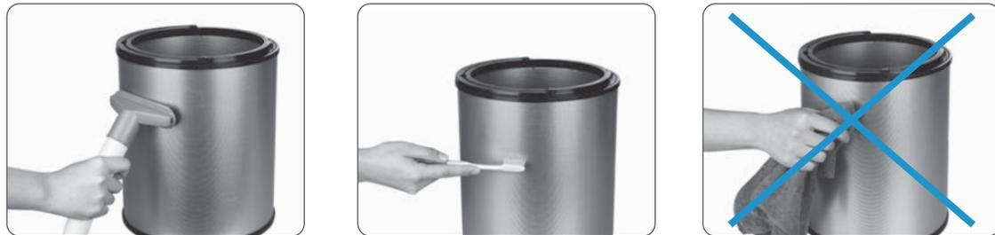
To clean the pre-filter, remove the two carbon barrels. Clean off the dust on the outer surface of the carbon barrel. Please carry out this procedure outdoors. Reinstall the carbon barrels, and press the "Reset" button in the respective controller interface to confirm.
