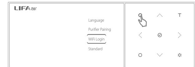
Press and hold "⚙️" on the monitoring controller to enter the main menu, touch "⏏️" to move selection box to "WiFi Login" and press "⏏️" to confirm.
